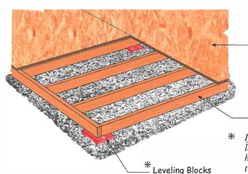
*Optional Floor:* Constructed with treated 2x4 framing. Floor joists are spaced 16" on center and covered with 5/8" OSB (oriented strand board).
