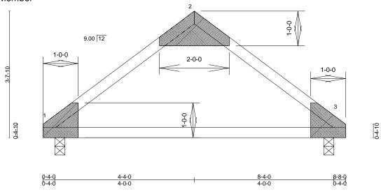
Attach Bottom Chord To Wall Top Plate with (1) Simpson H2.5A Hanger Both Ends of Truss
