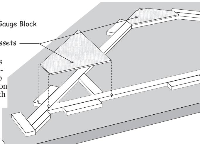
8. Repeat process to assemble (6) six more trusses. Do Not remove the 2x4 blocks around the perimeter of the truss until the gables are assembled in the next step.
