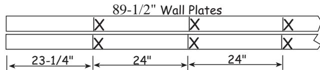
2. Install pre-cut wall studs between the top & bottom plates.
