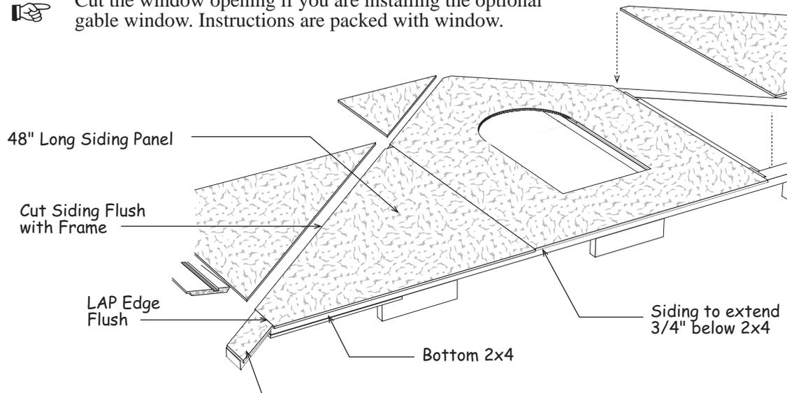
4. Cut siding and install on the ends of the gable. The siding should extend 1/2" below the 2x4 to receive the soffit when installed later.
