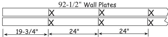
2. Install pre-cut wall studs between the top & bottom plates. Nail studs to wall plates with 10d sinkers, (2) two nails on each end.
