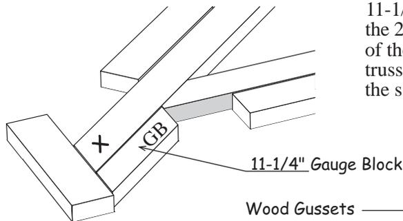
6. Install wood gussets to secure truss parts in place. Apply wood glue between gussets and 2x4s. Secure top gussets with (12) twelve 6d common nails. Secure the lower gussets with (16) sixteen 6d common nails.
