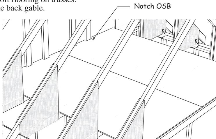
2. If necessary, cut flooring to the center of the 2x4.
