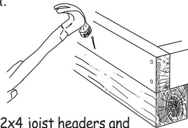
Nail 2x4 joist headers and floor joist to 4x4 runners.
