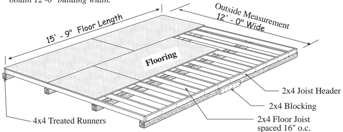
It is important that the floor be level and square. Square the floor as follows: before nailing the flooring, measure the floor diagonally (corner to corner). Then measure the opposite corners; these measurements will be the same when the floor is square. Toenail frame to the 4x4 runners.
