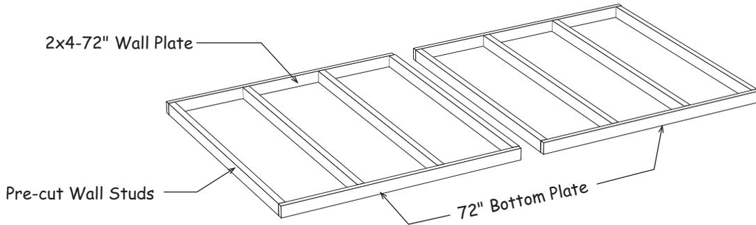
2. Install pre-cut wall studs between the top & bottom plates. Pre-cut wall studs will be 92-5/8" or 92-1/4" in length. Nail studs to wall plates with 10d sinkers, (2) two nails on each end.
