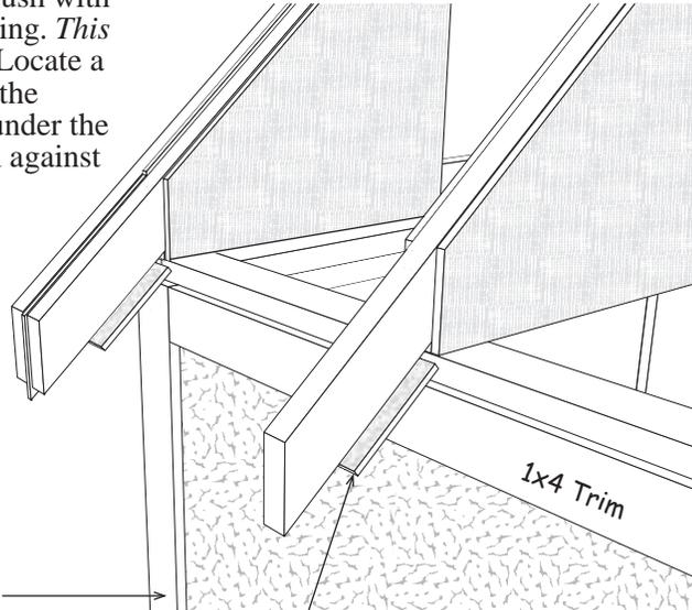
6. Starting from back gable install a 4'x10-5/8" soffit panel with bevelled edge. Cut the length so the panel ends at center of 2nd truss. Insure bevelled edge is facing truss ends. Use 6d galv. nails.
