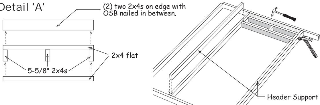
3. Secure the header by nailing through the top plate and wall studs with 10d sinkers.
