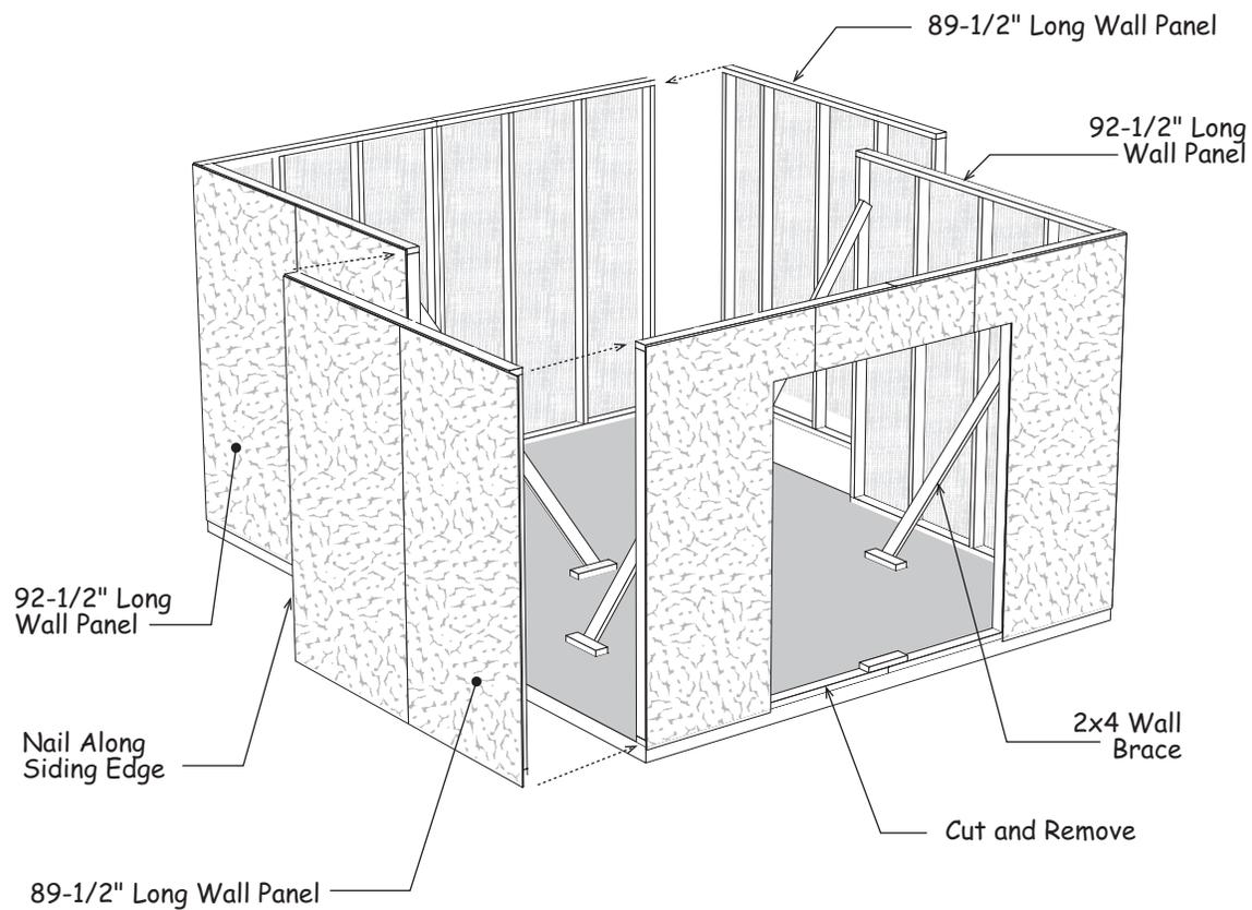
6. Cut and remove the bottom 2x4 in the door opening.
