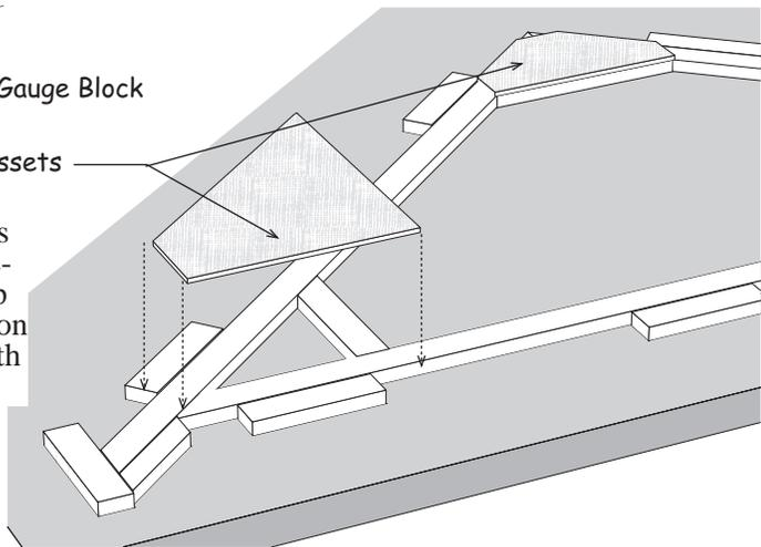
8. Repeat process to assemble (8) eight more trusses. Do Not remove the 2x4 blocks around the perimeter of the truss until the gables are assembled in the next step.
