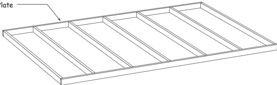
2. Install pre-cut wall studs between the top and bottom plates.
