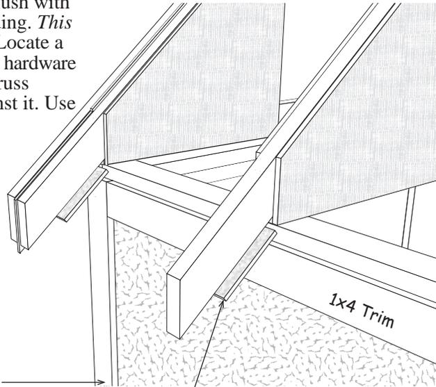
6. Starting from back gable install a 4'x10-5/8" soffit panel with bevelled edge. Cut the length so the panel ends at center of 2nd truss. Insure bevelled edge is facing truss ends. Use 6d galv. nails.
