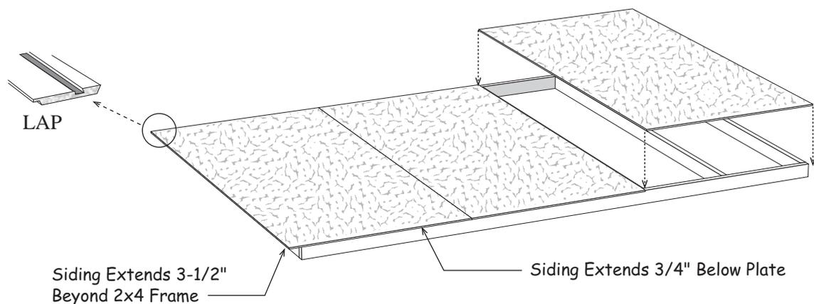
6. Repeat to apply siding to the other sidewall frame.
