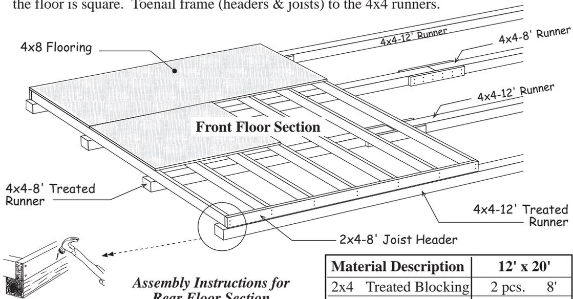
6. Cut (2) two 2x4-12' to a length of 11' -9 ". Layout for 16" joist spacing, *See above*.
