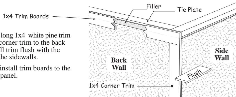
3. Install 95" long 1x4 white pine trim boards as corner trim to the back wall. Install trim flush with the siding on the sidewalls.
