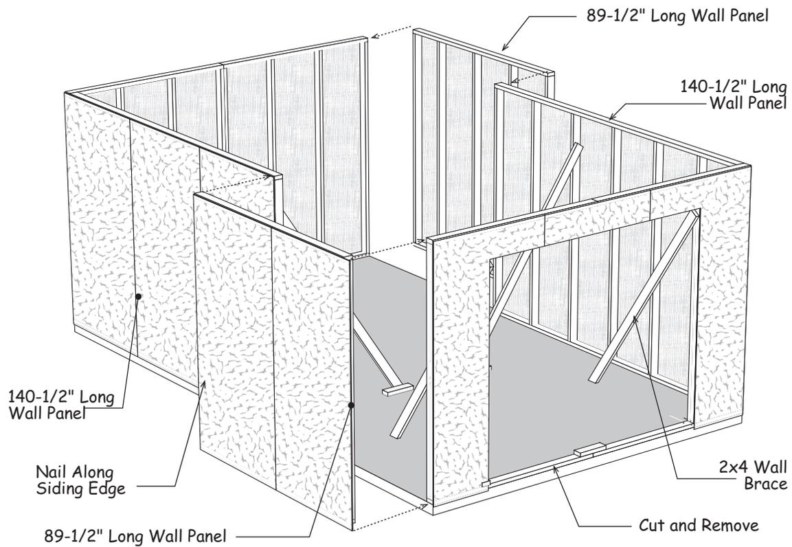
6. Cut and remove the bottom 2x4 in the door opening.
