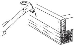
Nail the 2x4s to the 4x4 runners to keep the 2x4 frame from moving.
