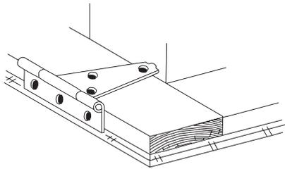
1. Lay the left door with the trim facing up. The siding on the left door extends past the door trim. See detail below.
