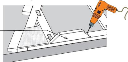
5. Turn the gable over. Locate pre-cut gable siding. Starting from left install the siding extending 3/4" below the bottom 2x4. Insure the siding does not extend above the top frame. Use 6d galv. nails spaced 12" apart.
