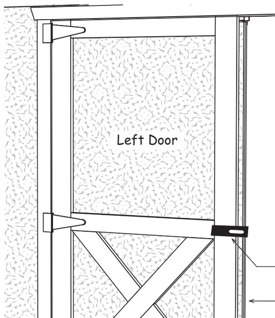
4. Before you fasten the hinges to the door trim, temporarily prop the doors in the opening. Leave a space at the top of the doors and between the doors and the side trim to allow room for the doors to expand when they absorb moisture.
