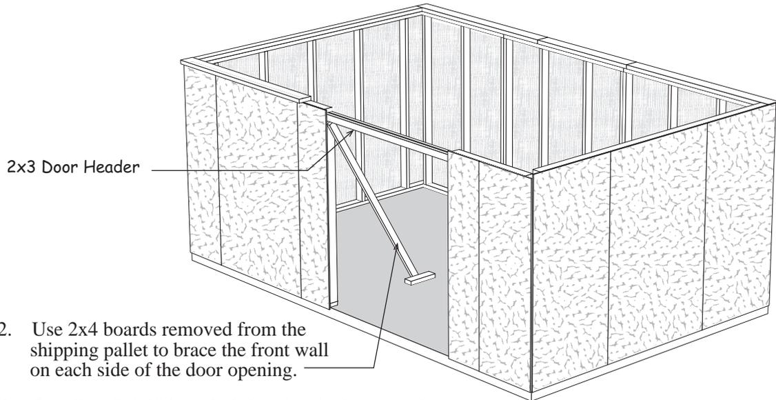
2. Use 2x4 boards removed from the shipping pallet to brace the front wall on each side of the door opening.
