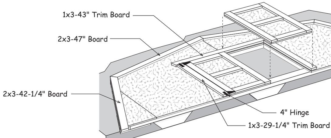
5. Apply 1x4 trim to gable. Install a 47-1/2" long 1x4 at the top of the gable. These boards have a blue marking on one end. Install this end at the top. Install trim flush with the top of the gable frame. Use 6d galv. nails.
