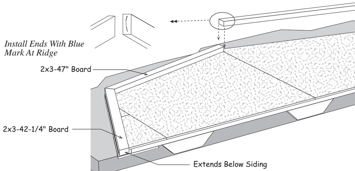
3. Apply 1x4 trim to gable. Install a 47" long 1x4 at the top of the gable. These boards have a blue marking on one end. Install this end at the peak. Install the 1x4 gable trim extending 1/2" above the siding on the gable. When installed later, the roof sheathing will be flush with the top of the trim.
