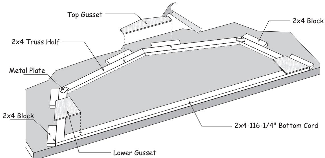
7. Assemble another truss without a bottom cord. Locate wood gussets with a 2x4 block attached to one side.
