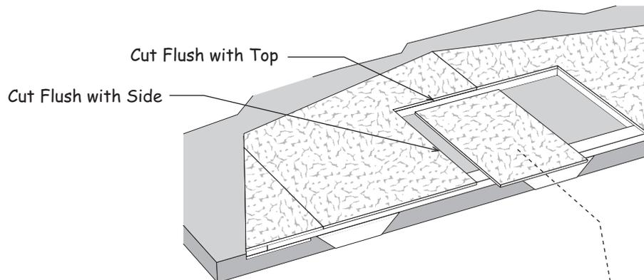
3. Assemble the loft doors. The loft door frames are temporarily held together with corrugated fasteners, this is the back side of the door frame. Place the doors on level surface, face side down. Cut the siding from above step to the size of the door frame. Secure the siding panel to the frame with 1" screws provided.
