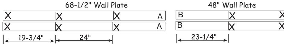
2. Install 72" wall studs between the top and bottom plates. Assemble frames and nail together with 10d sinkers.
